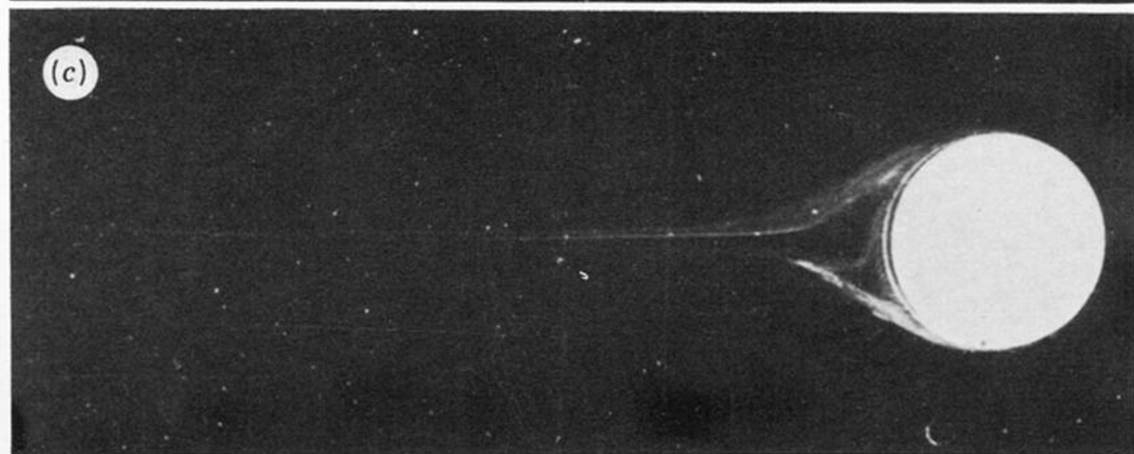
FIGURE 19. Plan photographs illustrating the increase in separation bubble size with increasing R_0 for f -plane flow with Ek = 13.8 \times 10^{-4} and R/H = 0.73 .
